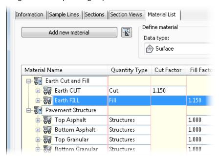
Quantity reports are created from a sample line group and can be inserted in a drawing as a table, or extracted to an external file. After a quantity report is created, if the corridor model changes, the section data attached to the sample lines also updates. When the section data attached to the sample lines updates, the quantity table in the drawing also updates. This makes it very easy to quickly analyze quantities and adjust corridor models to balance earth cut and fill volumes.
