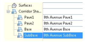
Standard names are assigned to subassembly shapes. For pavement structure, the convention is Pave 1, Pave 2, Base, and SubBase. The name in the criteria is a generic reference to the material name.
