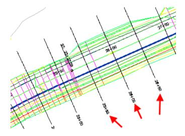
Earth cut and fill, and pavement structure quantities, are calculated from data associated with cross sections at the sample lines in order to estimate the amount of earth to be moved and the required materials for construction. Earth cut and fill volumes are calculated by comparing the corridor datum surface section data with the existing ground surface section data. Pavement and base material volumes necessary to construct the roadway are calculated directly from the corridor section data.
